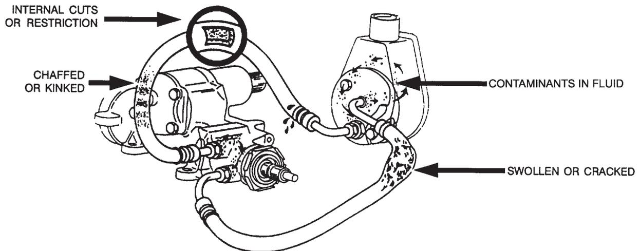
**Note:** CONTAMINATED FLUID COULD CAUSE THE SAME SYMPTOMS. ALWAYS FLUSH THE ENTIRE SYSTEM AND INSTALL A POWER STEERING FILTER.
