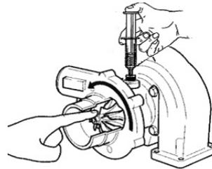
3. The engine oil and filter(s) must be changed before starting the engine. Use only a grade of oil approved by the OEM manufacturer for your specific vehicle/application. Some units have a micro screen filter inside the oil supply fitting that must be checked for contamination. Service or replace the screen as necessary.
