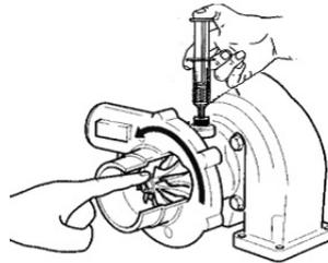
3. The engine oil and filter(s) must be changed before starting the engine. Use only a grade of oil approved by the OEM manufacturer for your specific vehicle/application. Some units have a micro screen filter inside the oil supply fitting that must be checked for contamination. Service or replace the screen as necessary.
