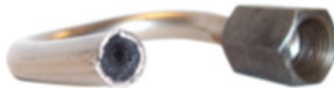
Cut-away showing blocked oil line
